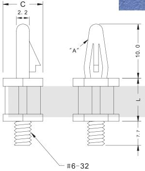
"A" HOLE IN P. C. B Ø 4. 0 P. C. B THICKNESS 1. 6
