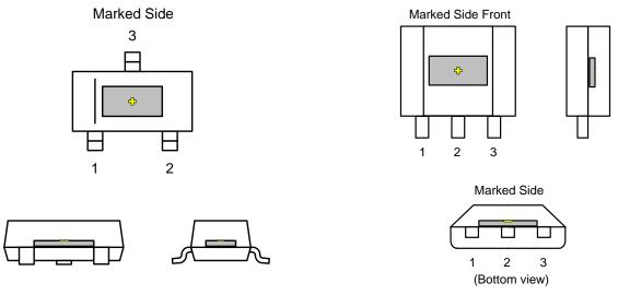
Figure 25. SOT-23 (DBZ) Package
