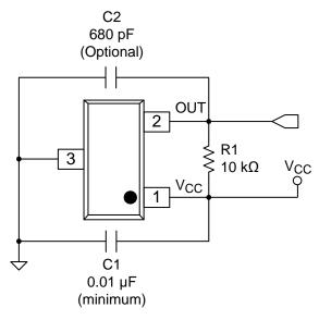
Figure 18. Typical Application Circuit
