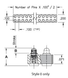
**Description:** Interconnect SLC Header Spring-Loaded Header Vertical Mount SMT Double Row Surface Mount **Plating Code:** Shell Plating: 20μ" Gold over 100μ" Nickel Inner Spring Plating: 10µ" Gold
