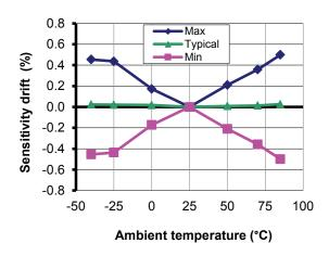
Figure 5: Sensitivity thermal drift
