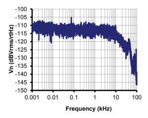
Figure 13: Typical noise voltage density of V ( $R_{\rm M}$ ) with  $R_{\rm M}$  = 50  $\Omega$
