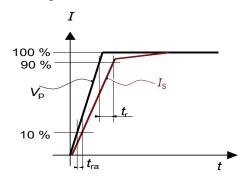
Figure 17: response time  $t_r$  and reaction time  $t_{ra}$
