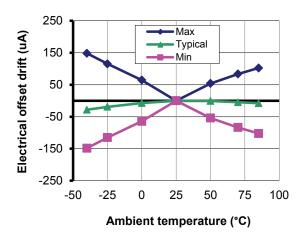
Figure 3: Electrical offset thermal drift
