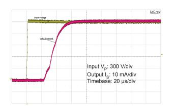
Figure 6: Typical step response (0 to 1500 V)
