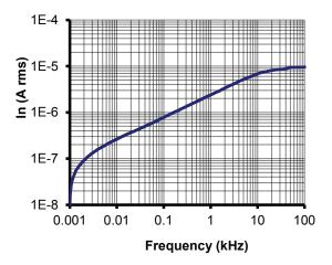
Figure 14:Typical total output current noise (rms) with  $R_{\rm M}$  = 50  $\Omega$  (fc is upper cut-off frequency of bandpass, low cut off frequency is 1 Hz
