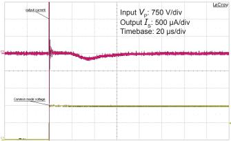
Figure 11: Typical common mode perturbation (1500 V step with 6 kV/ $\mu$ s  $R_{\rm M}$  = 100  $\Omega$ )
