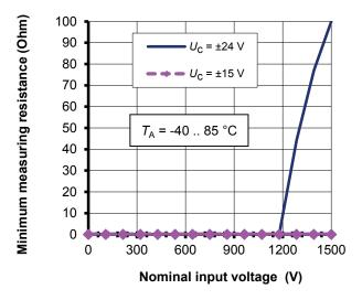
Figure 2: Minimum measuring resistance For  $T_{\rm A}$  under 80 °C, the minimum measuring resistance is 0  $\Omega$  whatever  $U_{\rm C}$
