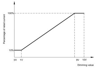
10V PWM signal for output current adjustment (Typical): Frequency range:100HZ ~ 3KHz
