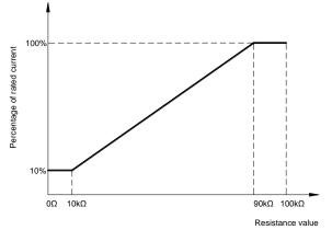
1 ~ 10V dimming function for output current adjustment (Typical)
