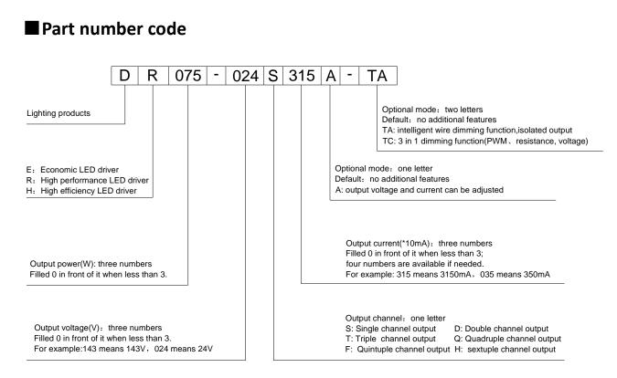
For example: DR075-024S315A-TA means: high performance LED driver; output power 75W; output voltage 24Vdc; output current 3150mA; single output; output voltage and current can be adjusted; with intelligent wire dimming function and isolated output.
